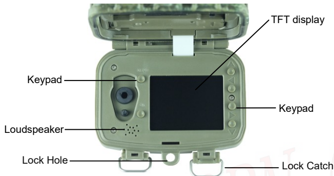
Figure 1.3: Display Screens and buttons view of Ltl-6210MC PLUS
